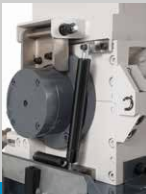
Piston assists raising and lowering steel cutting chamber cover.
