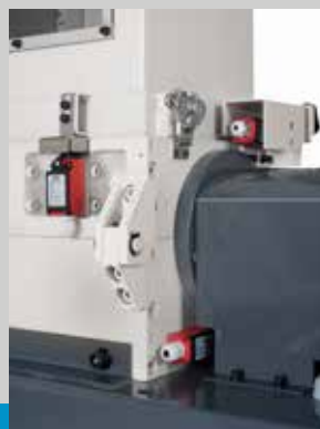
Multiple safety switches ensure cutting chamber is disabled during maintenance.
